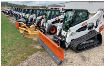
Figure 1. Terrestrial example of a modular disconnect system that allows the exchange of implements for a single mobility platform in-situ. [1]
